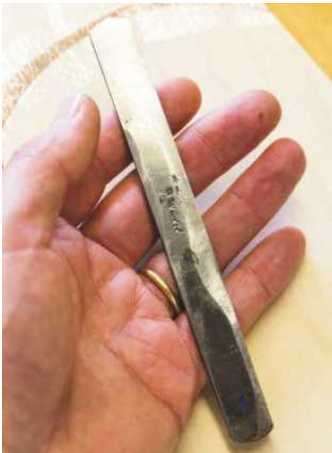
Another Japanese tool, this time a knife, whose high-carbon steel takes an excellent edge, and flat back suits it beautifully to cutting veneers following a deep guide
